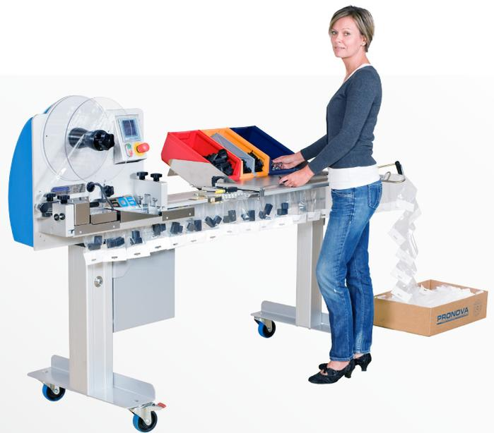
The Pronova 505 bagging machine is the smallest model in our range of standard machines. With a simpler design and fewer components than the other machines in the 500 series, it is particularly well suited for smaller growing productions that have packed manually into single bags and need to develop the packaging process to become a little more automated and much more efficient.
